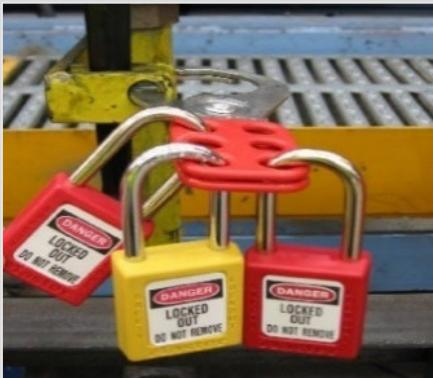
Note: Out-of-service tags or yellow locks may also be used to identify an isolation supervisor and left in place for the duration of the job. If this is the case, then the isolation supervisor needs to also use a personal (red) isolation lock when working on the electrical equipment
